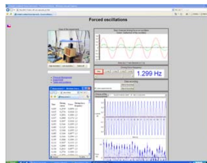
FIGURE 5 THE WEB PAGE OF THE REMOTE EXPERIMENT OSCILLATIONS WITH LIFE WEB CAMERA VIEW (TOP LEFT), GRAPH OF THE TIME REPRESENTATIONS AND CONTROLS
