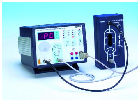
Fig. 7: Commercial laboratory device „Franck-Hertz experiment“ by Phywe (left), which is used in remote experiment developed by iSES Remote Lab SDK (right). http://194.160.213.12/index_js.html on PŘF UKF Nitra, http://147.251.193.82/index.html on Ped MUNI in Brno.
