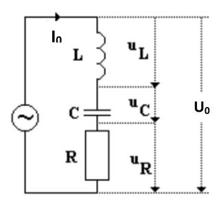
Fig. 1: Schematic of the RLC circuit
