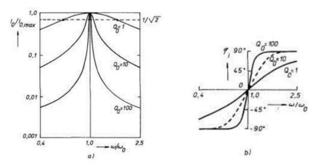
**Fig. 2**: Reduced resonance curve and reduced frequency dependence of the phase angle of the series resonant RLC circuit.
