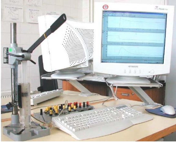
Fig. 9 Experimental setup with ISES for the measurement of the change of the state of the real gas
