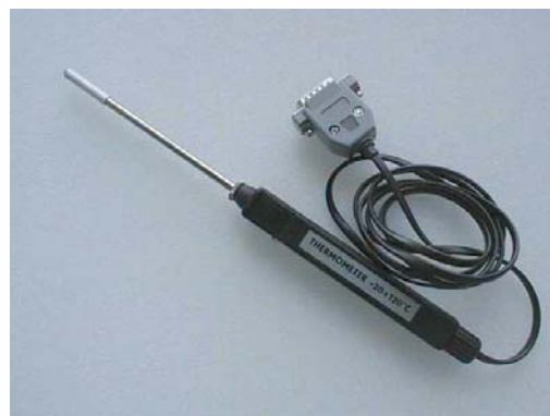
Fig. 3 Temperature sensing module the range -20^\circ\text{C} \div +120^\circ\text{C}
