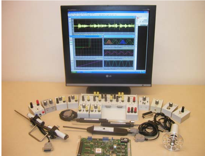
Fig. 1 ISES: The hardware with the main panel, interface card and incomplete set of modules
