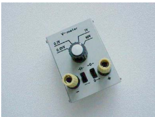
Fig. 2 Module for voltage measurement the range \pm 5\text{mV} \div 10\text{V}
