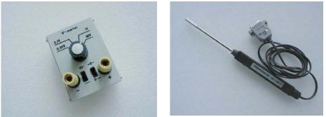
$\begin{array}{c} FIGURE \ 2 \\ \mbox{Module for voltage measurement} \\ \ The range \pm 5 \ mV{\div}10 \ V. \end{array}$
