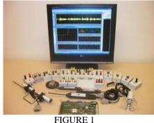
INTERNET SCHOOL EXPERIMENTAL SYSTEM (ISES): THE HARDWARE WITH THE MAIN PANEL, INTERFACE CARD AND INCOMPLETE SET OF MODULES
